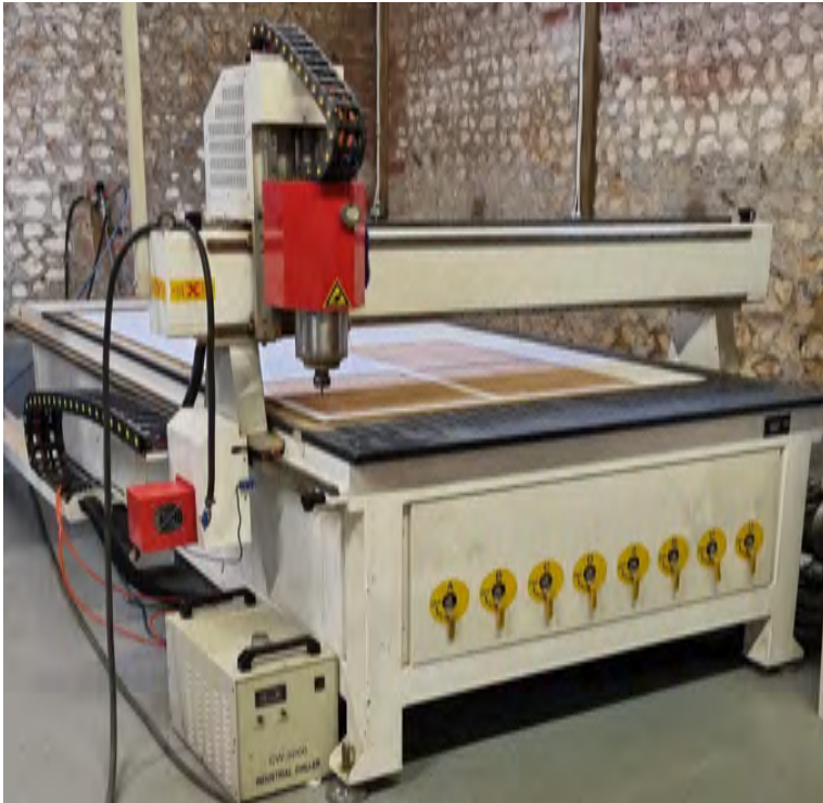
Large bed router used for precision machining of the 12 -25mm thick composites
