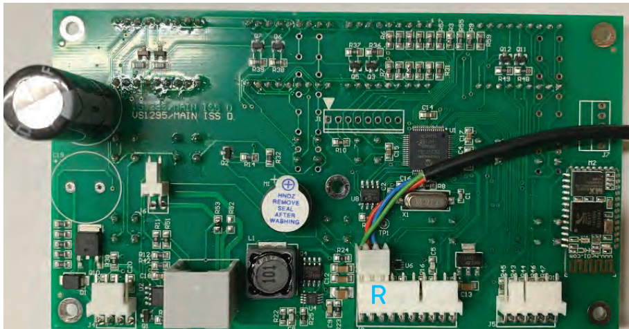
R Rotor recognition Pins 1,2,3
