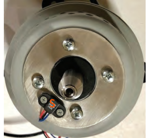
S Rotor recognition sensor
